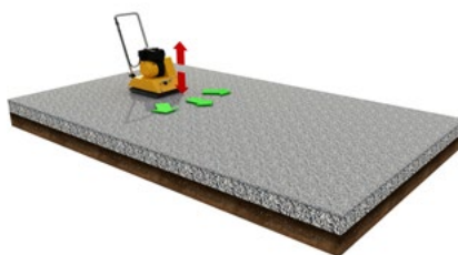
5. Proceed with the compaction of the surface layer
