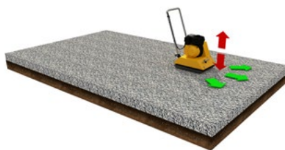
2. Surface compaction and levelling
